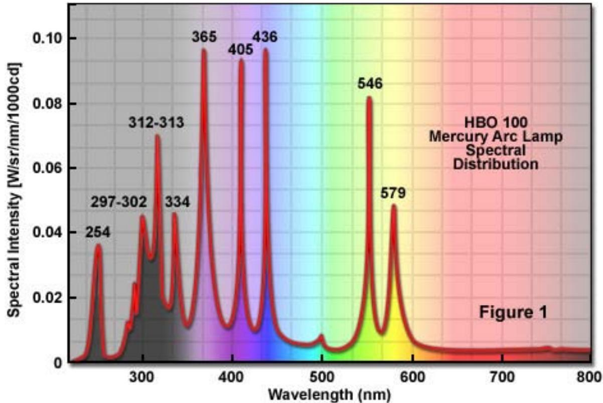
*Zeiss-Campus, Fundamentals of Mercury Arc Lamps*
